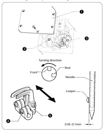
The loopers run in back of the needles in their forward travel and in front of the needles in their backward travel. Adjust the clearance between the needles and the loopers to anywhere from 0.05 to 0.1 mm in the forward travel.
