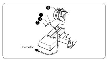
Connect the ground wire to the sewing machine head and motor.
