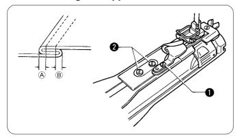
Insert the lapper guide plate from the front into the oval slot in the forward feed arm cover, making sure that the end of lapper is clear of the presser foot.
