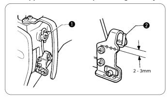
Adjust the distance between the center of the upper thread take-up and the top of the thread guide will be  $2 \sim 3$  mm.
