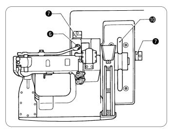
3. Place the machine head on the table, adjust its position in forward and backward directions by aligning it with the hole for presser bar lifter chain **6**, and in sidewise directions by aligning it with belt hole **10**.
