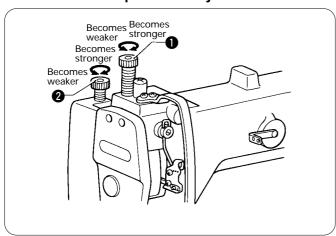
Adjust the presser foot pressure by turning presser adjusting screw • so that the pressure is just enough to feed the work positively and keep the work from slipping.
