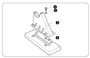
2. Place pulley cover A 3 so that it is in between the eight pulley cover seats 5, and then secure it to the pulley cover base with the four screws 4.
