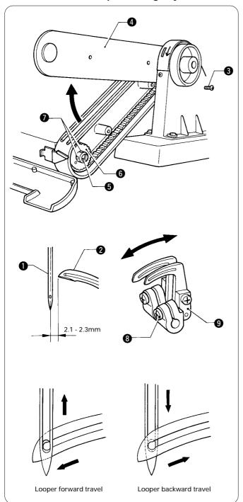
Make an adjustment so that, when needles ① are down lowest loopers ② reach the end of their backward travel and the distance from the needle center to the looper tip is 2.1 to 2.3 mm.
