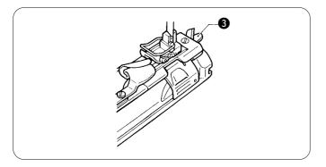
5. After sewing the work, move the work to thread cutter 3 to make blank stitches, and cut the thread with it.
