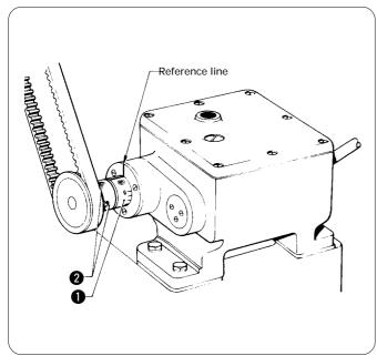
Make an adjust so that, when the needle bar is down at the lowest position, the mark on timing collar • is in line with the reference line.
