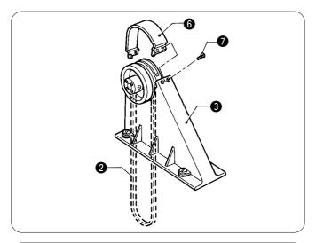
3. Push the belt 2 downward, and then install pulley cover B 6 to pulley cover A 9 with the three screws 7.
