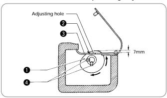
Make an adjustment so that, when the loopers begin moving backward, lower thread take-up ① contacts thread ②, and is 7 mm up from lower thread take-up base ③.
