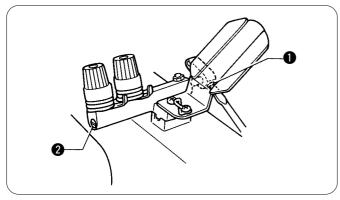
Adjust the thread release shaft so that the thread tension discs loosen when the presser foot is raised and tighten when the presser foot is lowered.
