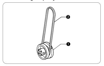
1. Place the belt ② onto the machine pulley ①.
