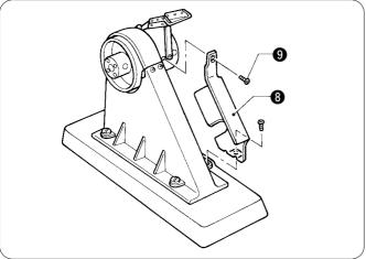
4. If the machine is being used with the puller attached, install the puller belt cover 3 with the two screws 9.
