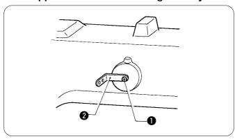
Adjust the upper thread arm thread guide so that the upper thread has a slight tension when the loopers run out of upper thread loops.
