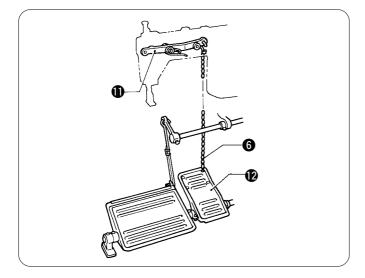
5. Connect the presser bar lifter chain **3** to the knee lifter lever **1** and the presser lifter pedal **2**.
