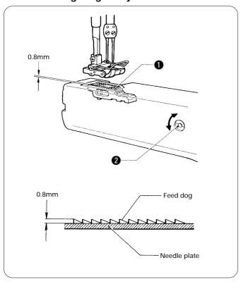
Adjust the height of feed dog • so it is 0.8 mm above the top of the needle plate when feed dog • is at the highest position.
