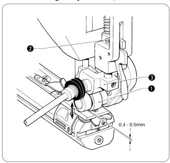
Adjust the height of puller **1** so that it is 0.4 to 0.5 mm high from the top of the needle plate.
